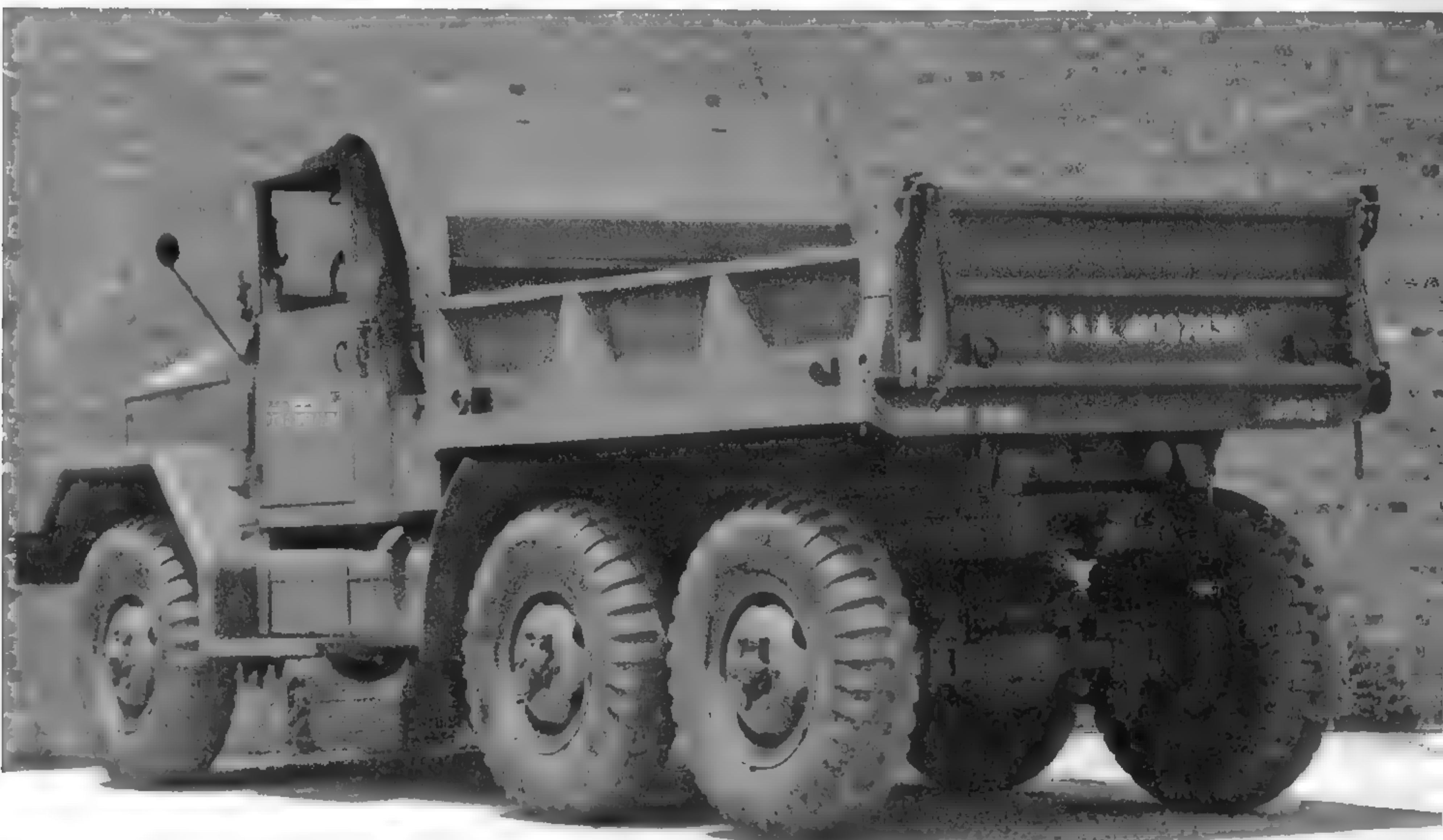
Like the M275, the M47 used the long fuel tank on the driver's side in place of the standard passenger's side tank. (Photo courtesy of the Patton Museum)
